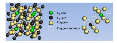
The scheme of the cubic structure of  $Y_2O_3$  and the schematic representation of  $C_2$  and  $S_6$  sites of  $Y_2O_3$ . (*See for example: D. Avram, B. Cojocaru, M. Florea, C. Tiseanu.* <u>Advances in luminescence of lanthanide doped  $Y_2O_3$ : case of  $S_6$  sites</u>. Opt. Mater. Express. 6(5), 1635-1643 (2016))
